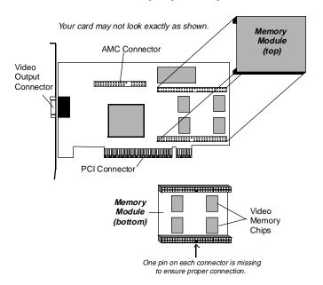
When installing memory module, use care to ensure that every pin is properly seated and the module is correctly oriented. If you are unsure of this procedure, please contact a professional technician to aid in the installation.
