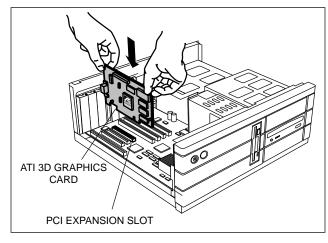
5 Replace the screw to fasten the card in place, and replace the computer cover.
